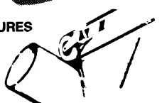
Grind radius with belt over shaped contact wheel
