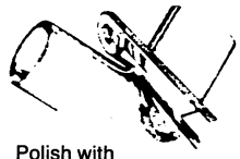
Polish with unsupported part of belt
